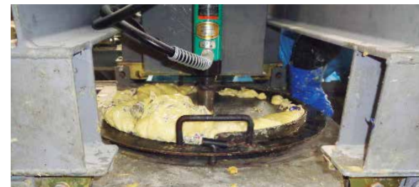
Machine for separating cheese and aluminum
