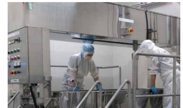
Test operation at a small-scale plant (curd stirring and whey removal equipment)
